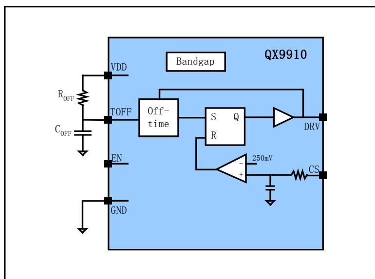
The  $T_{OFF}$  can be reduced by adding  $R_{OFF}$  and be increased by adding  $C_{OFF}$ .
