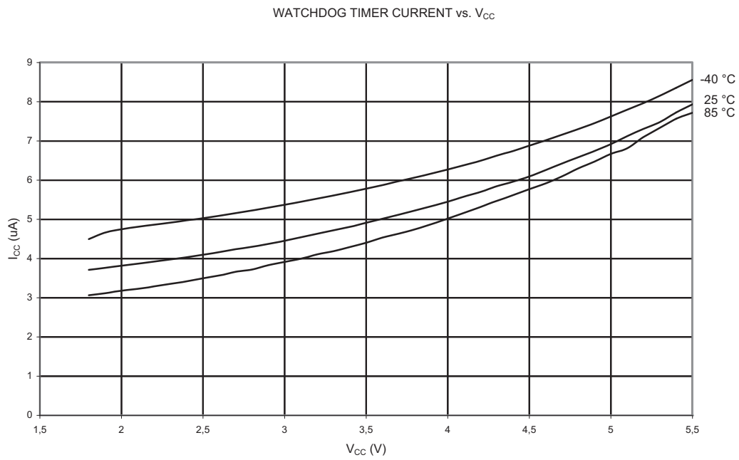
Figure 17-50. Watchdog Timer Current vs. V_{CC}
