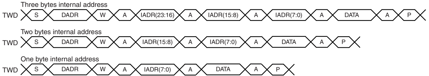
Figure 39-11. Master Write with One, Two or Three Bytes Internal Address and One Data Byte
