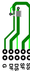
b. 125\text{ }^\circ\text{C/W} when mounted on a minimum pad of 2 oz copper.
