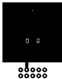
a) 55\text{ }^\circ\text{C}/\text{W} when mounted on a 1\ \text{in}^2 pad of 2 oz copper
