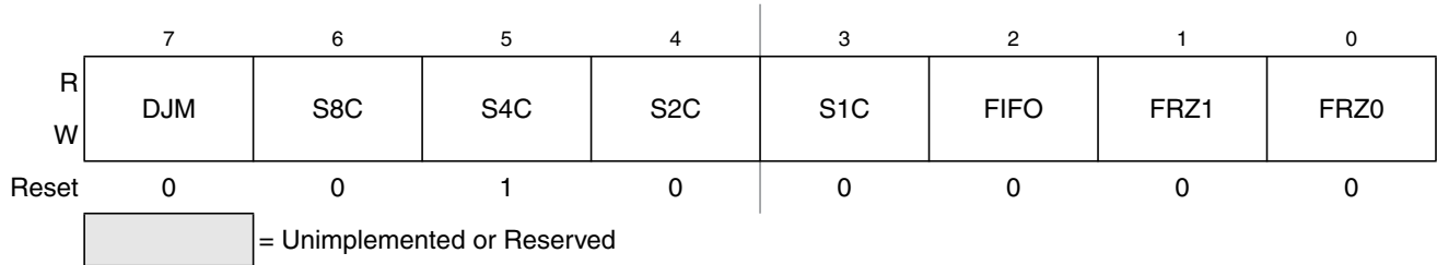
Figure 11-6. ATD Control Register 3 (ATDCTL3)
