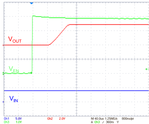
Figure 27: Enable transient ( I_{OUT} = 250 mA)
