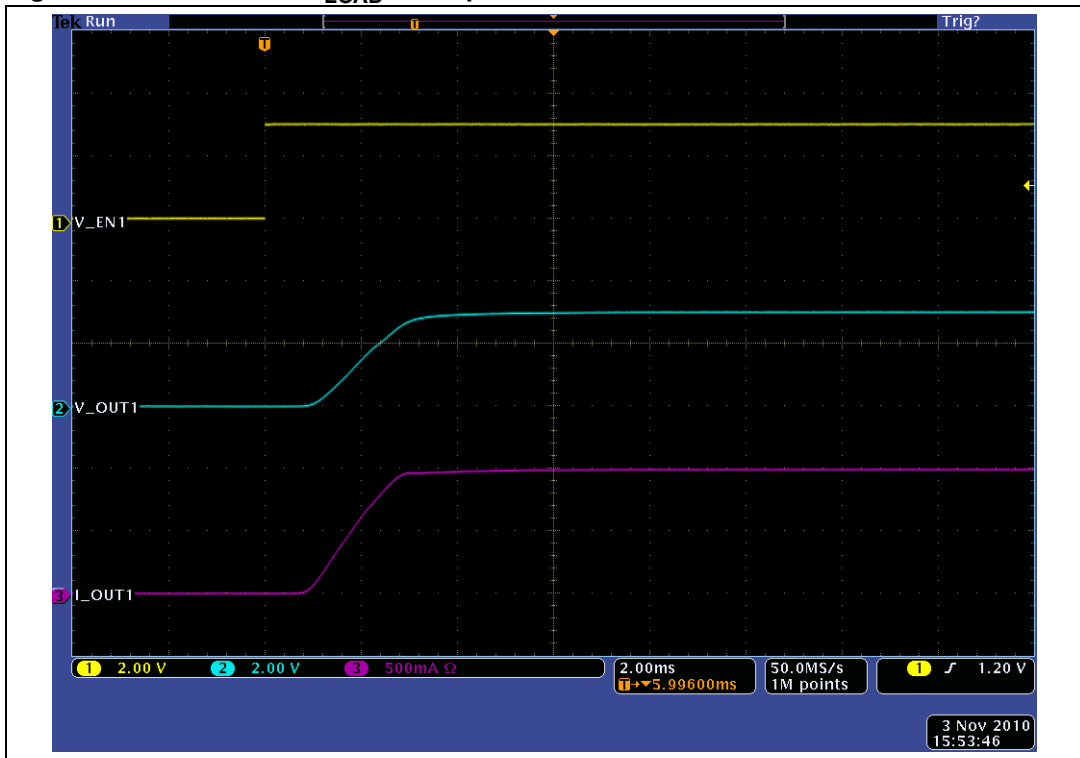
Figure 25. Turn-on for C_{LOAD} = 470 \mu F
