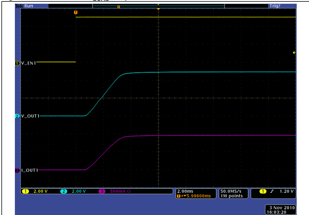
Figure 29. Turn-on for C_{LOAD} = 1 \mu F
