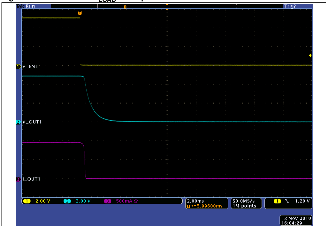
Figure 33. Turn-off for C_{LOAD} = 100 \mu F
