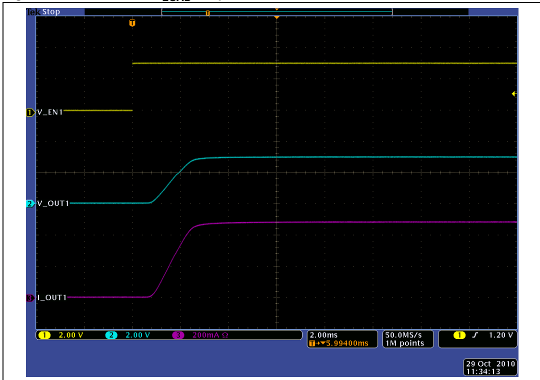
Figure 3. Turn-on for C_{LOAD} = 1\ \mu\text{F}
